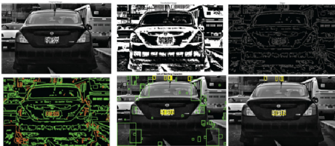
Fig. 8. Example of the step by step process to extract the characters as shown in Fig. 2. First, potential locations of the plate are found. Once the algorithm determines the right location, the characters are extracted.
